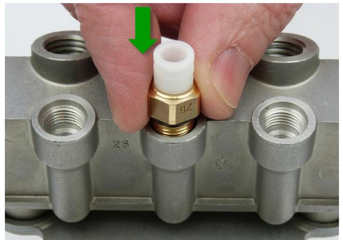
Fig. 12: Positioning the assy at right angles
