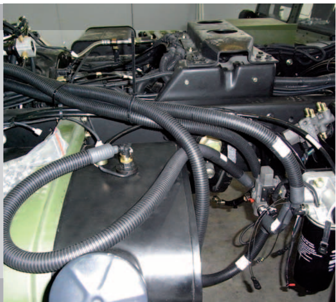
Prototype mounting of electrically heated fuel lines
